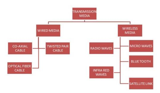
**Wired Media**- It includes various types of cables which are used to transfer data over computer networks.
