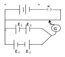
9. Two cells of emfs $\mathcal{E}_1$  and  $\mathcal{E}_2$  ( $\mathcal{E}_1 > \mathcal{E}_2$ ) are connected as shown in figure When a potentiometer is connected between A and B, the balancing length of the potentiometer wire is 300cm. On connecting the same potentiometer between A and C, the balancing length is 100cm. Calculate the ratio of  $\mathcal{E}_1$  and  $\mathcal{E}_2$ .
