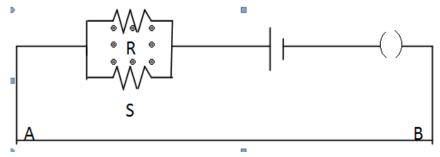
8. In a potentiometer circuit, a battery of negligible internal resistance is set up as shown to develop a constant potential gradient along the wire AB. Two cells of emfs $\mathcal{E}_1$  and  $\mathcal{E}_2$  are connected in series as shown in the combination (1) and (2). The balance points are obtained respectively at 400cm and 240cm from the point A. Find (i)  $\mathcal{E}_1 / \mathcal{E}_2$  and (ii) balancing length for the cell  $\mathcal{E}_1$  only.
