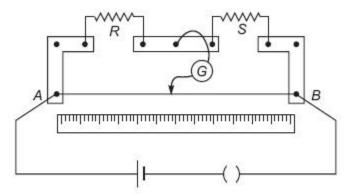
14. In a meter bridge, the null point is found at a distance of 40 cm from *A*. If a resistance of 12 <sup>[2]</sup> is connected in parallel with *S*, the null point occurs at 50<sup>[2]</sup> 0 cm from *A*. Determine the values of *R* and *S*.
