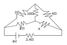
12. Find the value of the unknown resistance X and the current drawn by the circuit from the battery if no current flows through the galvanometer. Assume the resistance per unit length of the wire is  $0.01\Omega \text{cm}^{-1}$ .
