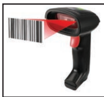
Figure 1.8: Capturing Data using Barcode Reader
